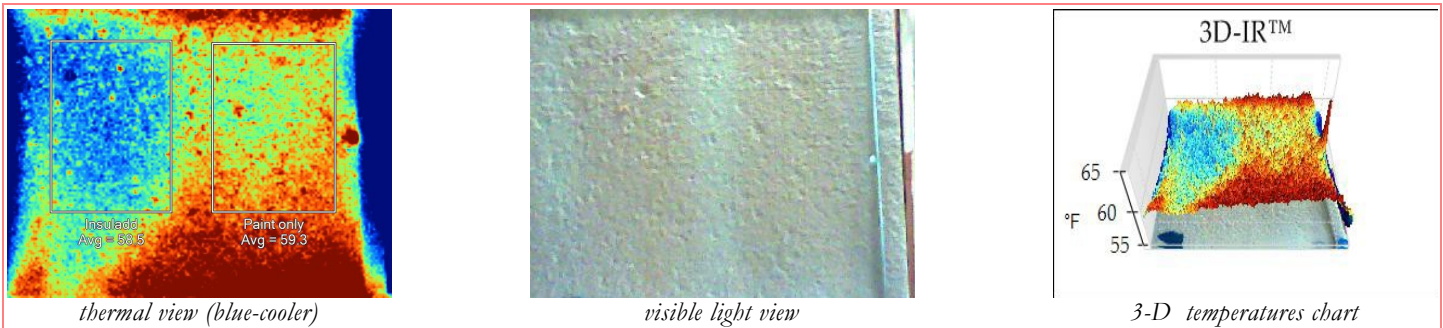
Heated foam box side-by-side comparison of Insuladd® (inside left /blue-cooler) to paint-only (inside right/red-green)
