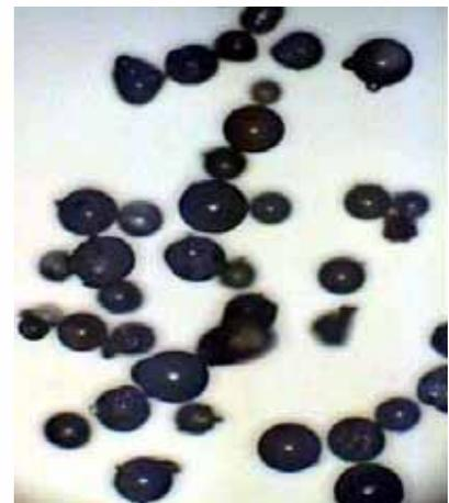
The powder was examined under a stereo microscope which showed that the material is spherical in nature as is depicted in the photograph above right... see the 500 times magnification of Insuladd®.
